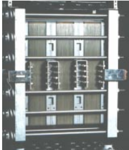
(from top) Redox-flow battery Micro gas turbine undergoing field test
